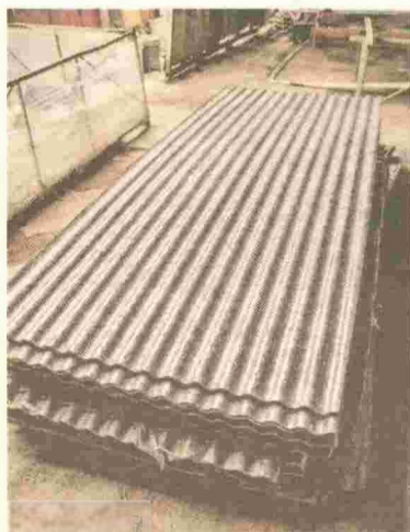
The finished product — Poly-Al roofing sheets.
